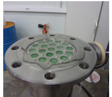
Bubble test: sealing test integrity of housing, membranes and gaskets
