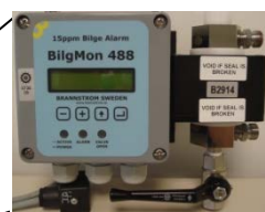
15 ppm Oil alarm monitor
